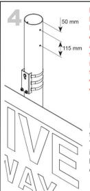
Important: Mark and drill 4 holes Dia 10mm (2 each side) at 50mm and 165mm from the top of the post in such a manner that the solar panel will face due South when fixed.
