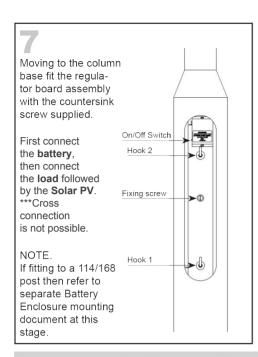
Take the battery packs and hang 2 from the lower hook 1 on the regulator board. Connect the batteries to the battery connectors.
