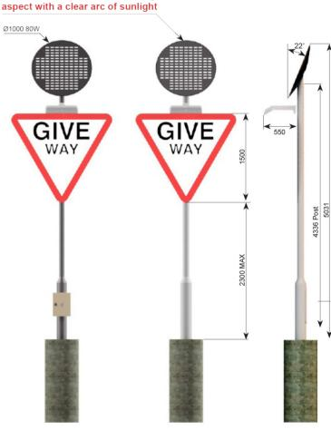
114 / 194 Post with Internal **Batteries**
