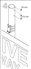
Important: Mark and drill 4 holes Dia 10mm (2 each side) at 50mm and 165mm from the top of the post in such a manner that the solar panel will face due South when fixed.
