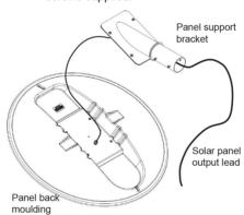
Fix the sign to be illuminated to the post in its final position. Mark and drill a 14mm cable entry
