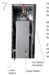
Hang the battery pack from the hook below the regulator. Connect the battery to either of the available battery connectors.
