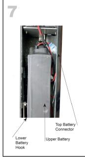
Fit the lower battery hook shown at the fixing point with M8 hex socket set screw and nuts supplied. Take the first battery pack and hang from this hook using the extension loop supplied. This will position the battery in the lower position. Connect the battery to the longer battery connector.
