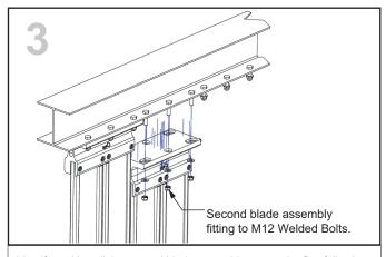
Identify and install the second blade assembly next to the first following the same method outlined in step 2.
