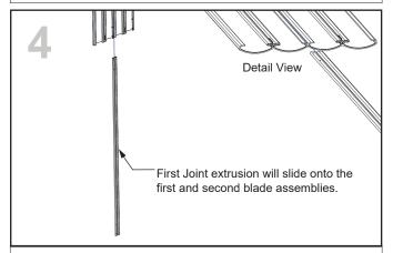
Join the first and second blade assemblies by sliding the first extruded joint strip bridging the first and second blades.
