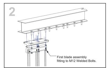
Identify the first blade assembly and carefully remove the joint strip and retain the four fixings.
