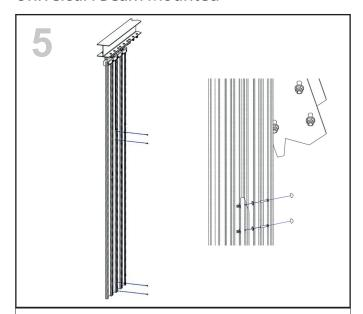
Join the first and second blade assemblies with the first joint strip and fix with the four retained fixings.
