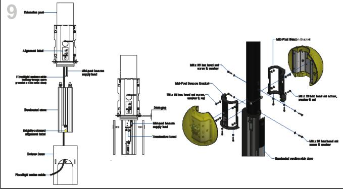
Unpack the extension post, uncoiling the 1.5mm<sup>2</sup> lantern mains cable tucked inside the bottom. Note: The other end of the cable is under the reducer cap. This cap should be removed before fitting the lantern.
