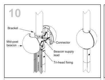
Connect each half of the mid-post beacon to each end of the beacon supply lead and hook the vertical studs on the beacon halves onto the holes at the top of the brackets. The bracket has been supplied lightly clamped only, and will need to be tightened up at this point, ensuring it remains correctly aligned.
