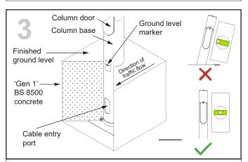
Insert the column base into the hole, making provision for the mains supply to enter the base through the cable entry port.
