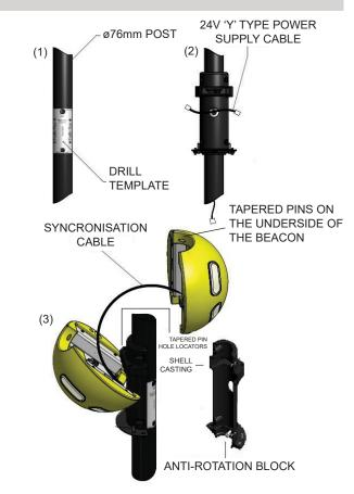
the cable from the beacon into the output lead of the transformer. Coil any excess cable in the base compartment and tie up neatly.
