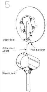
Pull the solar output lead out of the solar panel support bracket and carefully lift the solar panel assembly above the solar panel spigot. Connect the solar output lead to the PV connection lead using the corresponding plug and socket.
