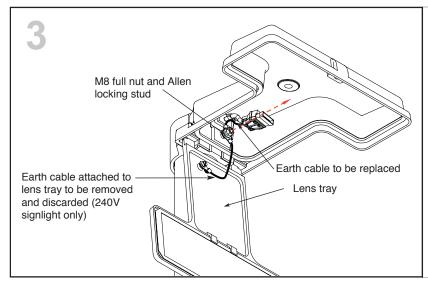
With the existing light unit removed, disconnect the two earth cables by releasing the M8 nut and removing the ring terminals on the locking stud.
