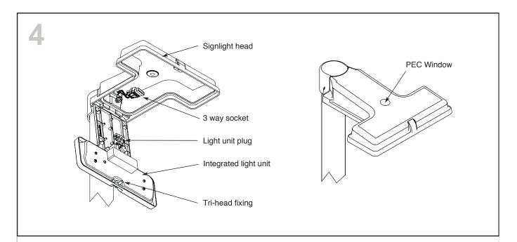
Hook the integrated light unit onto the signlight head as shown.
