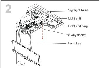
Remove the existing light unit by unplugging the 3 way socket and unlatching it from the signlight head. This is done by pushing the light unit back towards the post and at the same time pulling down gently.
