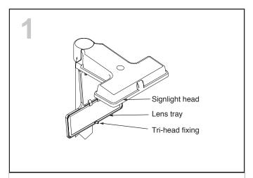
Release the Tri-head fixing and hinge the lens tray down.
