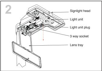
Remove the existing light unit by unplugging the 3 way socket and unlatching it from the signlight head. This is done by pushing the light unit back towards the post and at the same time pulling down gently.
