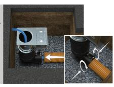
**7**Remove levelling pole once concrete is set.
