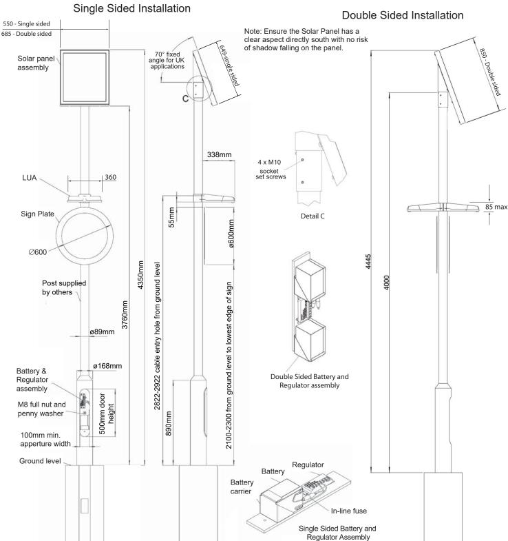
Install the post in line with the manufacturers guidelines, taking into account the type of soil, location and windage of the equipment being fitted.
