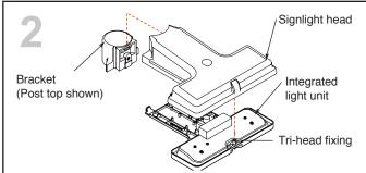
Remove the integrated gear tray by releasing the Tri- head fixing and hinge down gently before unhooking the tangs at the base. Be aware of any additional equipment that may be attached to the LUA body which will need disconnecting before the gear tray can be removed. Additional equipment will typically be remote monitoring nodes and certain photocells.
