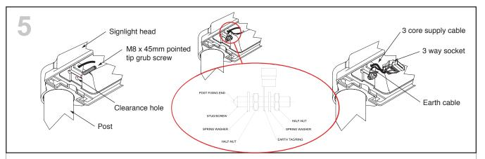
Take the M8 x 45 mm pointed tip grub screw and pass it through the clearance hole in the sign light head before turning it into the thread in the bracket. Using a 4mm Allen key tighten the grub screw sufficiently to prevent bracket rotation.
