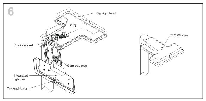
Use the tangs at the back of the integrated light unit to connect it back onto the signlight head.
