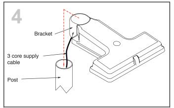
Feed the 3 core supply cable down into the post.
