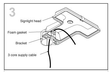
Feed the 3 core supply cable through the slot inside the bracket and on through the hole in the foam gasket at the back of the signlight head.
