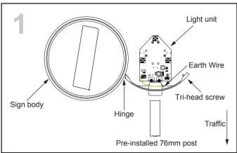
The Invinca Double Sided is designed to fit onto a pre-installed 76mm post.
