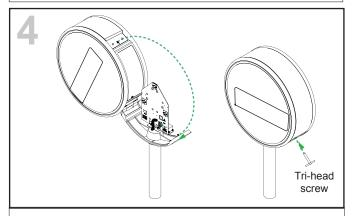
Refit the sign body to the hinge if removed earlier.
