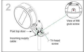
Using a Tri-head key, loosen the Tri-head security screw and hinge the sign body open.
