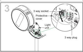
Remove the protective cover from the 3 way socket on the light unit and retain for use later.
