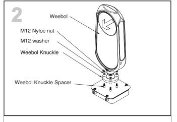
Remove the 4 x M12 Nyloc nuts and washers from the Weebol fixings in the centre of the adaptor plate. Place the Weebol over the 4 x fixings ensuring the 4 x spacers are in place. Check that the orientation of the Weebol is correct for the traffic application.
