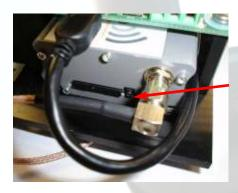
The Sim card holder is situated at the bottom of the modem.
