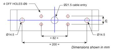
2. Mount the LU(M) onto the supporting structure. Two sets of fixing holes are provided to use a choice of either 4 x M8 or 2 x M12 A2 stainless steel fixings. The length of the fixings should suit the mounting structure and include A4 Stainless steel self locking nuts and penny washers. The fixings should be tightened to a torque of 15Nm if using M8 fixings and 60 Nm if using M12 fixings.
